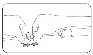
3. Connect the Power Cable to Male Connector of the Horti-Tube. And Twist the Cap.
