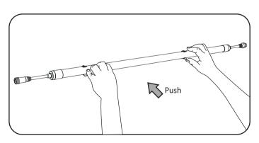
2. Pressing the Horti-Tube into the Clips.
