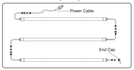
For Maxium Number of Tubes Connection per Power Cable. Please refer to Multiple Tube Connection Detail.
