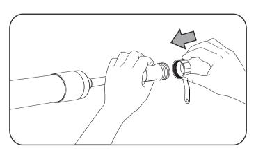
4. Twist the End-cap on the Female Connector.
